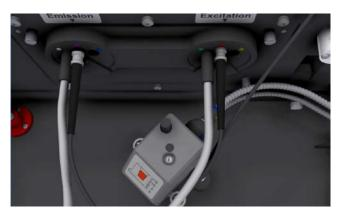
Figure 21: Turn the TRF optic head 45 degrees
