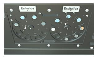
Figure 30: Filter change / filter installation: Loosen the filter wheel by loosen the nut in the middle (see text for detailed description).
