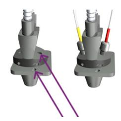
Figure 14: Holes to position reagent needles in the measurement head
