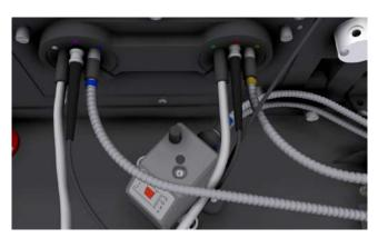
Fig. 23: Final look of the installed TRF optic head and light guides. Note: The excitation light guide must be positioned BELOW the black thin light quide of the absorbance spectrometer!
