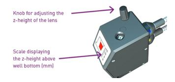
Figure 19: The TRF- optic head with z-height adjustment
