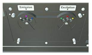
Figure 29: Filter change / filter installation: Loosen the 4 screws
