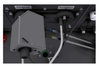
Figure 20: Feeding the light guides of the TRF-optic head
