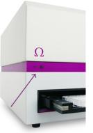
Press and hold the plate in / plate out button for 3 seconds, hereafter the plate carrier will automatically move to its lock position. Once the reader is switched off, the transport pin can be moved down and turned clockwise. The transport pin must be screwed until it tightens. Please tighten it firmly with your fingers. Don't use any tools.
