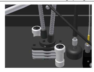
Figure 33: Example of spacers between measurement head and bottom of reagent box
