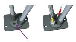
Figure 10: Holes to position reagent needles in the measurement head
