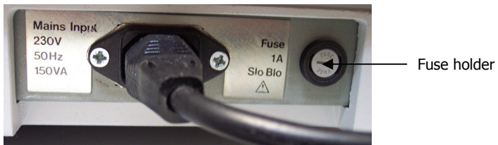
Figure 139 The position of the mains fuse
