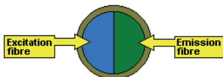
Figure 74 The end of the fibre optic accessory
