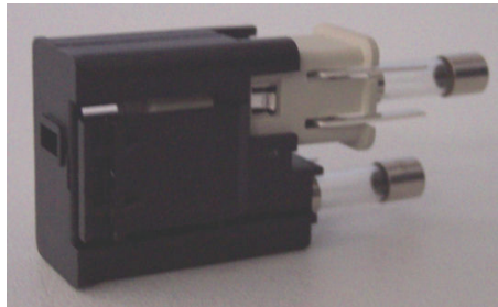
Figure 10 Fuse block removed from the PTP-1
